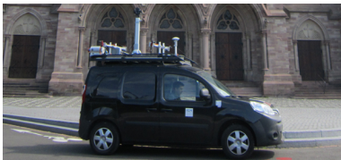
Figure: Stereopolis, IGN's mobile mapping system.
